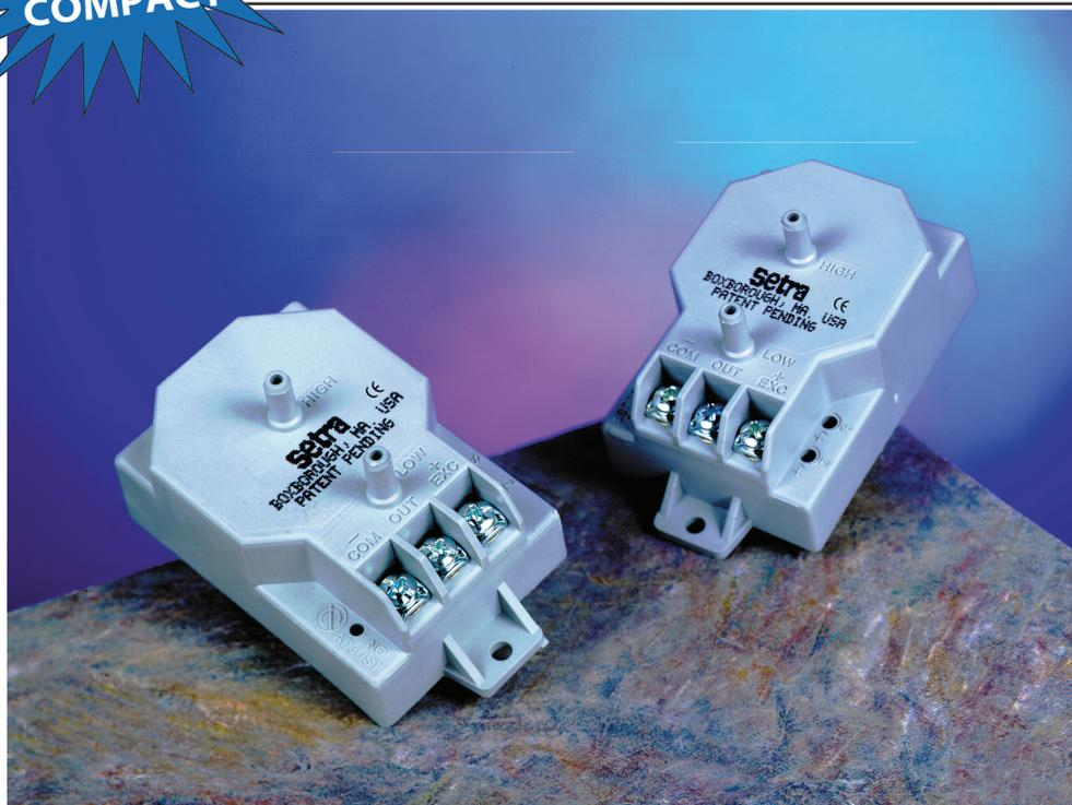
Setra Systems 265 pressure transducers sense differential or gauge (static) pressures and convert this pressure difference to a proportional electrical output. The 265 is offered with a high level 0-5 VDC output or a 4-20 mA output. It is also offered with 0-5 or 0-10 VDC output in the 24 VAC excitation version.
