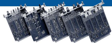
Expansion modules utilize a family of transceivers each designed to support a particular cable technology. Transceivers are identified by a suffix designation (e.g., -FOG) which follows the EXP model number. Each expansion module usually supports from two to four ports of the identified transceiver. Some expansion modules mix two cable technologies within one module minimizing the cost in some applications.
