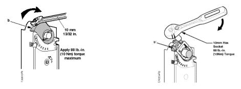
**NOTE:** Keep the shaft in the center of the shaft adapter opening.
