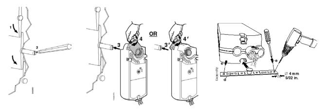
Figure 5. Finger Tighten the Actuator on the Shaft with the Damper Blades in the Desired Position.
