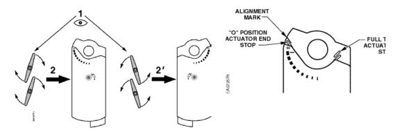
Figure 2. Actuator Mounting Orientation.
