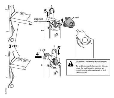
Figure 4. Shaft Length and Proper Shaft Adapter Location.
