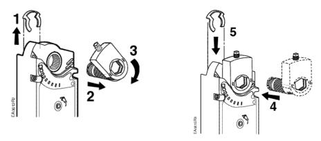
Figure 9. The Angular Rotation is Adjustable between  $0^\circ$  and  $90^\circ$  at 5 degree Intervals.
