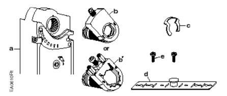
Figure 1. GGD Actuator Parts.
